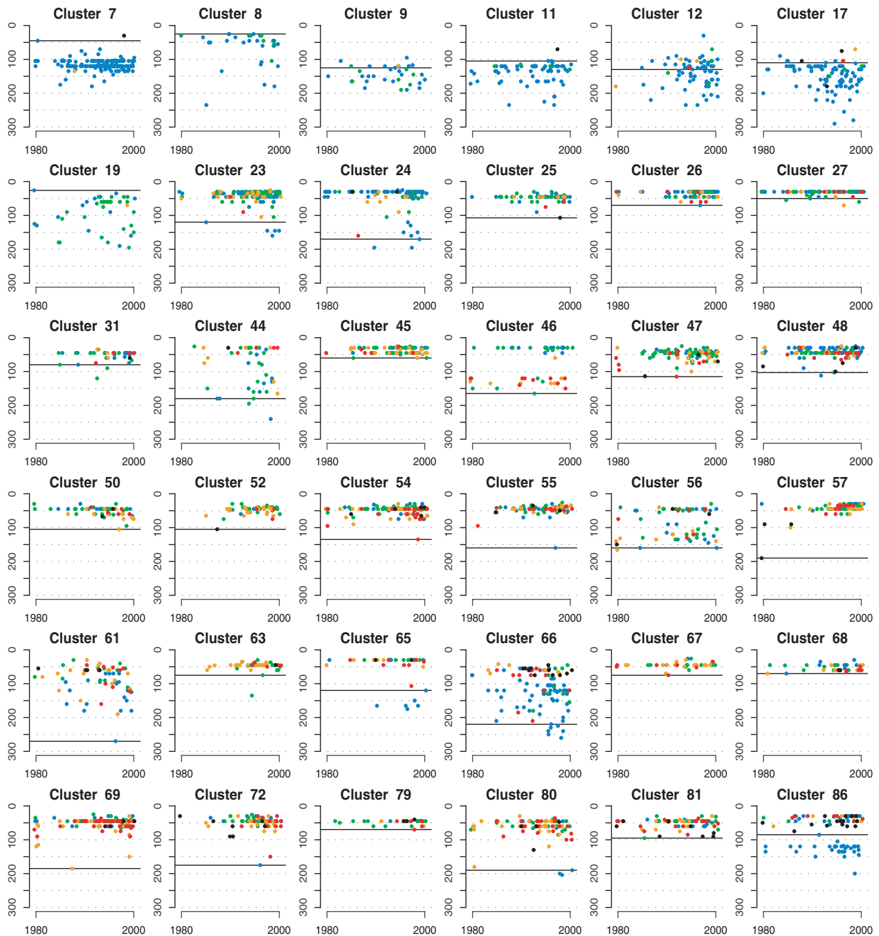
Fig. 4. Plots of arsenic level (indicated by color: blue, green, orange, red, and black, as in Fig. 1) as a function of depth and year of installation of well. (The relatively few wells installed before 1980 are assigned dates of 1980 in these graphs.) Data are displayed separately for each of the 66 spatial clusters (see Fig. 3). Each cluster is labeled by the average arsenic level of the wells in the cluster. The horizontal lines indicate estimated safe-depth thresholds (or lower bounds, where thresholds cannot be estimated), as described in Section 4.1 and mapped in Fig. 13.
